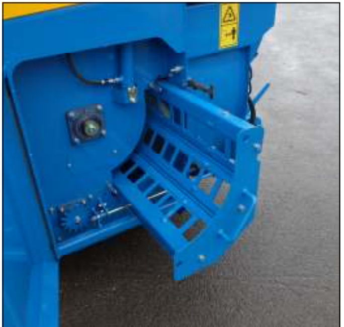
The unique beater, comb & concave will shred straw, silage, hay and short chop straw at variable lengths
