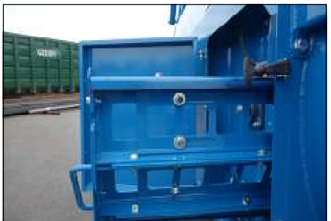
Adjustable concave screen louvers, vary chop length
