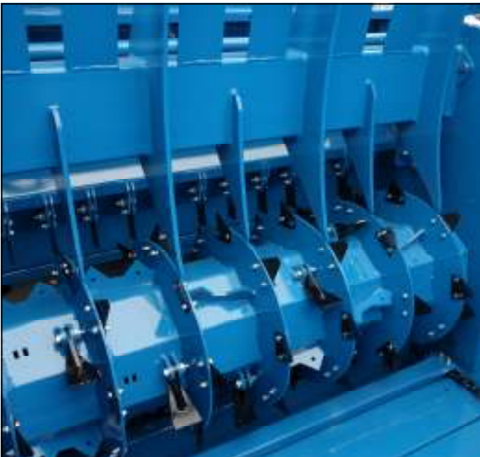
The unique beater, comb & concave will shred straw, silage, hay and short chop straw at variable lengths
