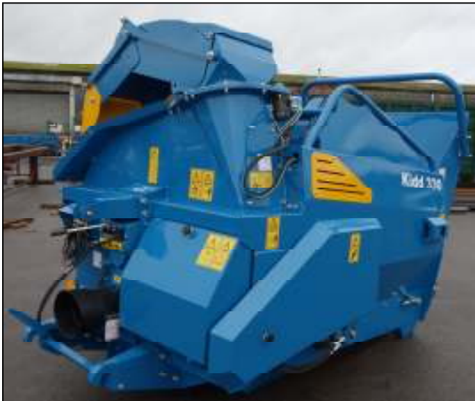
The 330 can be converted from mounted to trailed
