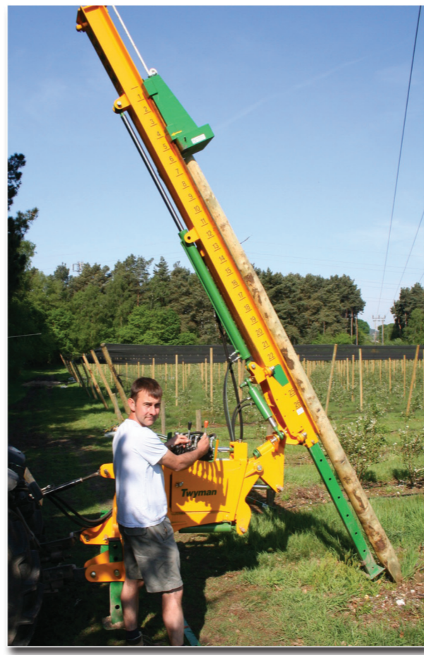
Drives posts into the ground from 30 degrees angle
