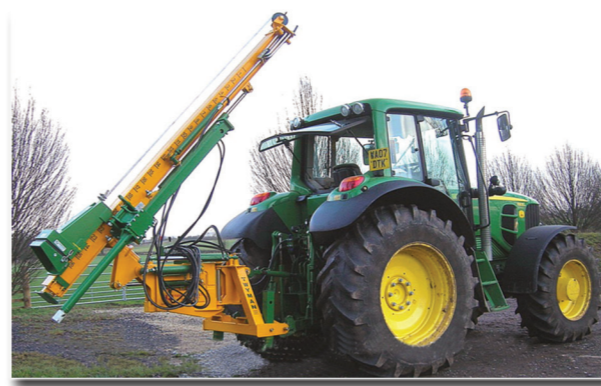
Despite the long mast for greater impact all post drivers fold neatly behind the tractor for transport
