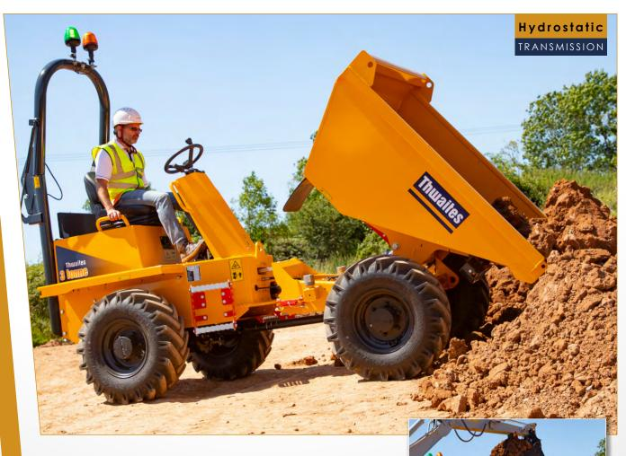
The Thwaites 3 Tonne Front Tip, Stage V dumper is manufactured with contractors and hirers in mind – ensuring operator safety, reducing risk on site and improving performance. Powered by an 18.1 kW 3-cylinder Yanmar engine, delivering 107 Nm max torque for optimum traction and control, this machine is driven by a Hydrostatic transmission, making it simple and straightforward to operate.
