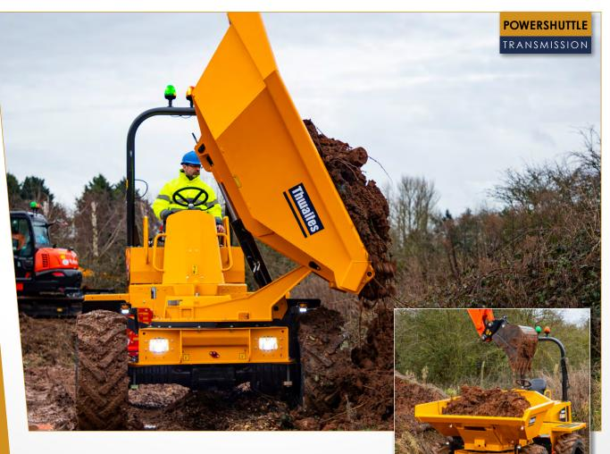
The Thwaites 6 Tonne Power Swivel, Stage V dumper is manufactured with contractors and hirers in mind – ensuring operator safety, reducing risk on site and improving performance. The Power Swivel skip enables a 90° rotation left and right, allowing the machine easier access to tip loads in restricted areas, giving the operator greater control and reducing risk on site.
