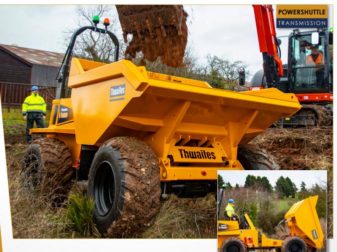
The Thwaites 9 Tonne Front Tip, Stage V dumper is manufactured with contractors and hirers in mind – ensuring operator safety, reducing risk on site, and improving performance. Front Tip dumpers allow the machine to be easily and safely unloaded, with a straightforward tipping action that places the full bucket of spoil exactly where it is required.
