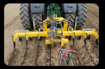
The legs are hydraulically lowered and raised without moving the main frame. This can be done on the move providing versatility of the loosening element of the machine in certain cultivation processes. The hydraulic front cutting discs allow complete versatility when using the machine in varying ground surface conditions, especially when experiencing surface trash. This is all achieved through one hydraulic service on the tractor.
