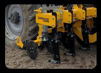
The machine wings are telescopic and have a locking position for transport. For field work the wing then slides out 0.5m to work as a 4m machine. The front cutting disc also slides in allowing the toolbar to fit neatly behind the tractor for transport.
