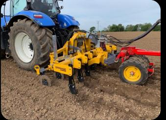
The machine is built with low disturbance legs and points which provide a full width lift with minimal surface disturbance. The front cutting disc enhances the loosening element of the leg and eliminates the surface tension, thus reducing any opportunity of soil boiling in front of the leg along with easing the flow of trash through the machine.
