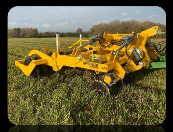
The 4 Metre Low Disturbance Loosener wings are hydraulic folding and can be adjusted into work and transport mode from the tractor cab. For field work, the wings unfold, interlocking into a rigid 4 metre machine and for road transport, the machine folds neatly behind the tractor and is secured with a locking bar.
