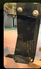
The machine is built with low disturbance legs and points which provide a full width lift with minimal surface disturbance. The front cutting disc enhances the loosening element of the leg and eliminates the surface tension, thus reducing any opportunity of soil boiling in front of the leg, along with easing the flow of trash through the machine.
