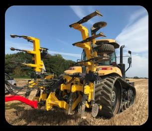
The 'Tight – Turn' system on the 6m toolbar ensures that the wings fold upward to 90 degrees automatically when the legs are hydraulically lifted out of work. This movement creates space for the operator to turn close to the trailing implement allowing for a 'Tight Turn' to be achieved on headlands.
