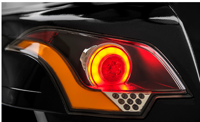
LED tail lights with brake lights and indicators
