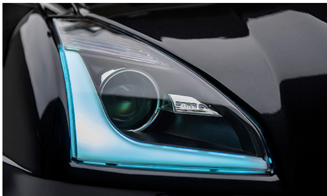
LED headlights with daytime running lights and high-beams
