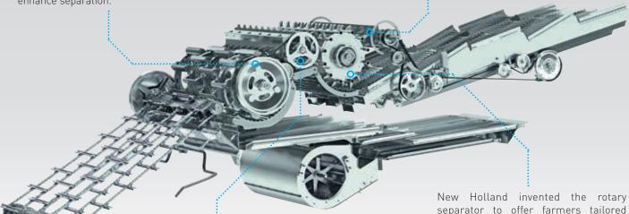
The beater's serrated teeth prevent mats forming in the crop to improve crop flow in all conditions, especially when harvesting marginal crops at high moisture levels.
