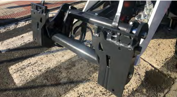
Quick-Tach™ to Bob-Tach™ adapter (required for all attachments except buckets and pallet forks)
